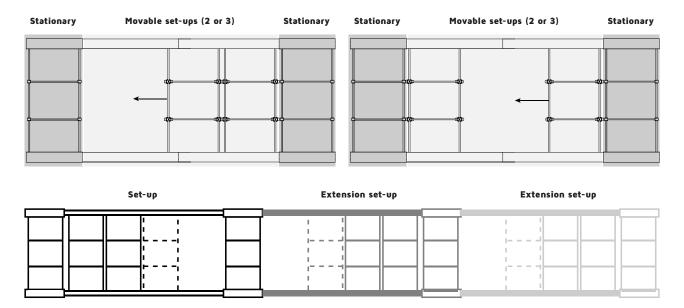
One UBeTrack $^{\text{TM}}$  can consist of 2 or 3 mobile shelves. The total width can vary, see the illustration below. This can be increased in 25 mm increments up to a maximum of 250 mm which in turn alters the width of the walkway.
